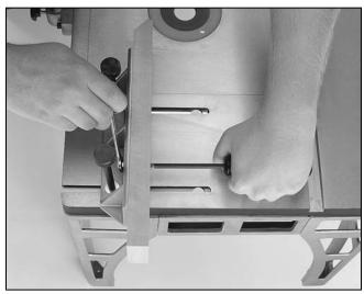
Figure 5. Attaching the wood facing.
